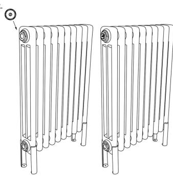
Insert the bleed into opposite top end cap of the radiator. The bleed should already have a gasket attached to it, if not, apply one of the spares. The bleed should now be tightened with an adjustable spanner, ensure the bleed is not over tightened.
