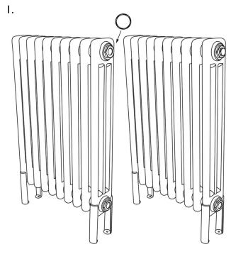
Insert the blank into desired top end cap of the radiator. The blank should already have a gasket attached to it, if not, apply one of the spares. The blank should now be tightened with an adjustable spanner, ensure the blank is not over tightened.
