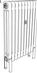
Attach the desired wall stay to the radiator. Please note that for radiators above ten sections, two wall stays will be required. A wall stay fitting guide can be obtained after purchase. Valves should now be attached to the bottom end caps of the radiator.
