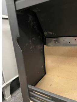
2. Remove left hand firebrick.
