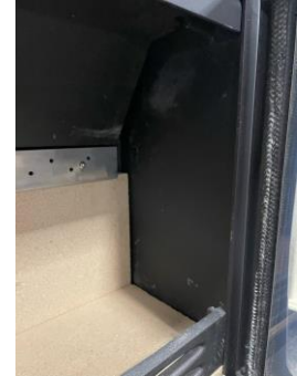
3. Remove right hand firebrick.
