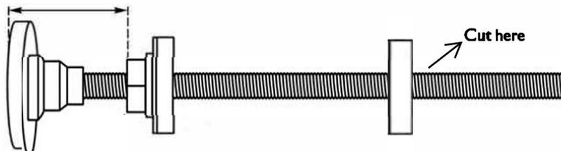
Measure the distance from the wall to where the back of the radiator is to sit, as shown above. The Clamping Plate can be used in either a vertical or horizontal position. Radiators with a smaller space between each section, the Clamping Plate should be positioned Vertically. Radiators with a larger space between each section, the Clamping Plate should be positioned horizontally. Install the red washer, then the Thistle head will screw through the un-threaded clamping plate.
