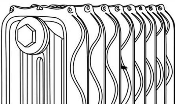
The radiator should now be moved into position, making sure that it is sat against the Clamping Plate.
