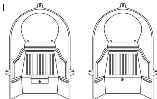
Remove the Firebrick Retaining Plate by removing the 1 x M6 Bolt, Washer and Nut.
