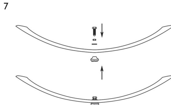
Attach the Ashpan Handle to the Ashpan using 1x M6 Bolt, 1x M6 Washer and 1x M6 Nut.
