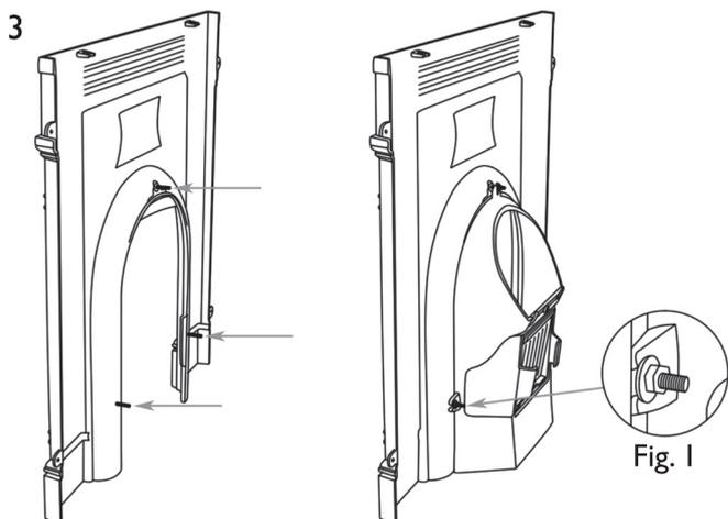
Insert the 3 M6 Studs into the back of the Fireplace Fascia. Attach Fireplace Back to the back of the Fireplace Fascia, ensuring that the M6 Studs pass through the fixing brackets on the Fireplace Back. Secure and tighten using 3 M6 Washers and 3 M6 Nuts, as Fig. 1.
