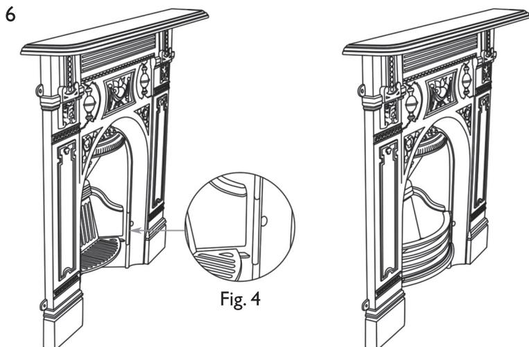
Slot the Bars through the grooves on the front of the Fireplace Fascia, as fig. 4.
