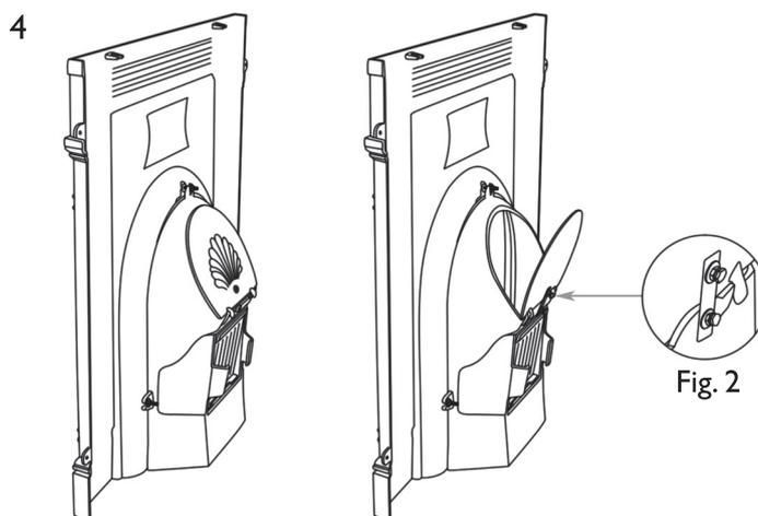
Solid Fuel Usage: Rest the Damper Plate onto the groove on the back of the Fireplace Fascia.
