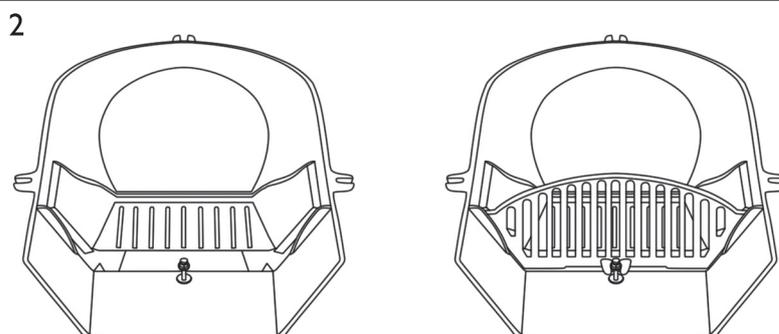
Lay Fireplace Back down on level ground. Position Firebrick in place and then insert 1 x M6 Bolt, passing through Washer and Nut, into the hole just below the Firebrick. Insert Grate into the groves on the Fireplace Back, passing the fixing lug over the M6 Bolt. Secure in place by tightening Bolt.
